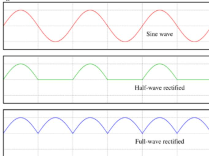
AC, half-wave and full-wave rectified signals.
